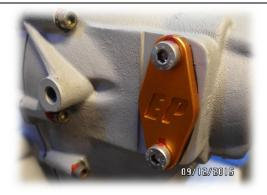
2. Clean the mating surface on the gearbox where the pump was attached with brake-cleaner, acetone or mineral spirit. Ensure the O-ring on the back side of the cover is in place. Install and tighten the included M8 socket head screws with the copper sealing washers under the bolt head to **14NM**.
