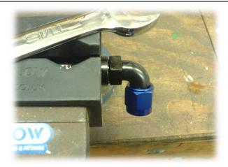
31. Keep torqueing until the hose end and the sleeve almost mates.
