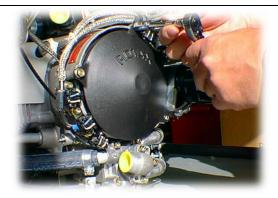
5. Remove the flywheel plastic cover by undoing the 3x 10mm M6 hex bolts.
