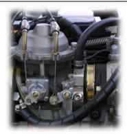
3. Now remove the LH/RH carburetors. Before you remove them, detach the air filters or airbox. Disconnect the choke and throttle cables. Disconnect the fuel hoses and hoses for coolant if you have carb heaters installed. Now loosen the Philips screw on the rubber socket flanges and firmly pull of the carburetors.
