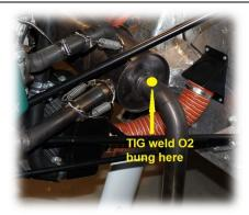
41. This picture shows the typical location of the O2 lambda sensor. The sensor is not intended to run on AVGAS. The sensor will correct the air/fuel mixture during low loads and normal operation, but not do any corrections on high loads. This ensures smooth running and optimal A/F ratio as well as a clean burning engine. NOTE — The engine will run just fine in case of a damaged or broken sensor!
