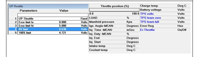
57. The TPS comes pre-set, but the idle set point may change as the user sets the idle stop. The TPS volts is displayed at the bottom of your screen. Read of the TPS volts at idle and insert the value in row 4. 0% limit. Next set full throttle and insert the TPS volt into row 5. 100% limit.
