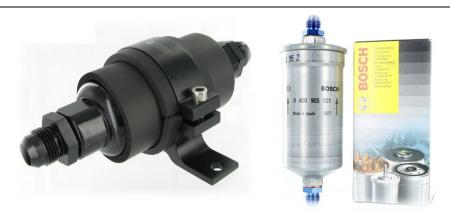
23. The <u>post-fuel</u> filter should be installed after the pumps. Note the arrow or in/out orientation indicating the direction of flow. Always try to install the filter in horizontal orientation. High flow, low restrictions or a gascolator is preferred prior to the pumps.
