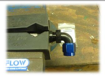
30. Clamp the assembly in the wise jaws and start to torque. Remember to lubricate the threads with some engine oil.
