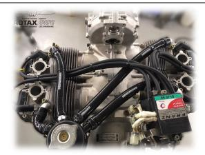
13. Replace the coolant hoses and re-orientate the coolant elbow on cylinder 1/2/4 as shown on the picture and install the 90° hose elbow cut to length. If you relocate the coolant elbows, use a M18x1 thread die and tap to clean the threads on the elbow and flange. Clean with Loctite Super Cleaner 7063 or mineral spirits, and re-assemble with Loctite 243 or 577. Torque the flange back onto the head with 10Nm. New upper coolant hoses with appropriate spring hose clamps are included in the kit.
