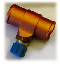
20. Cut the 25mm hose coming from the water collector tank, and install the coolant sensor adapter. It is usually convenient to use a 90° hose elbow. The "CLT" sensor is used for ECU engine temp feedback, mainly for cold or hot start, as well as enrichment when the engine runs hot.
