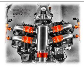
16. Install the 4-1 intake system on the engine. Ensure that the sealed off intake ports are free from any cloth, paper or plugs and insert new O-rings for the intake flanges. Orientate each intake flange with the mating flange on the cylinder heads.
