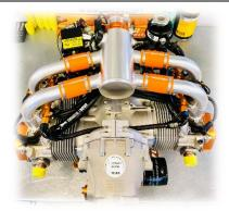
18. Cut the attached AN hose to length and make up the cross tube between the two fuel rails as shown on the picture above.
