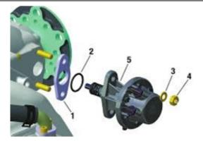
1. Remove the existing mechanical fuel pump. Start by removing the 6mm and 8mm fuel hoses. Remember to close the fuel valve before you start on this task. Next, remove the 2x M8 nuts and washers. Pull out the fuel pump and remove the isolator plate, gaskets and O-ring. Remove the M8 stud bolts by using a stud bolt extractor or simple by installing two nuts and unscrewing them.
