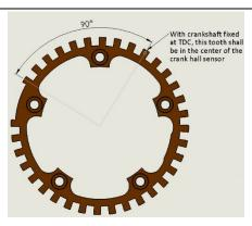
9. Install the crankshaft trigger wheel on the flywheel hub with the M5 bolts facing outwards. Apply engine oil on the flywheel bolt after cleaning it properly, and tighten the bolt to 45NM+180° or 32.2ft.lb + 180°. Install the hall sensor mount as shown above with the supplied 2x M6x25 socket bolts. Apply (Loctite 243) and tighten to 12NM. The yellow marked tooth shall be centered on the hall sensor with Cyl-1 at TDC, or with the crankshaft fixation bolt installed (PN 876-640)
