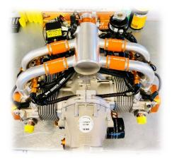
14. Picture showing a typical installation of the EFI system onto a Rotax® 912ULS engine.
