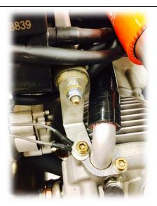
12. Terminate the two ignition grounding wires to the bracket bolt.
