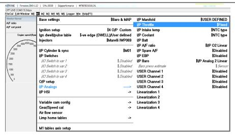
56. After starting the engine and setting the idle, go to M1, I/P Analogs and I/P Throttle. Now you can set the TPS idle and WOT limit. The TPS voltage is displayed in the picture as show in point 54.
