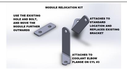
10. Install the provided relocation brackets for the ignition module. Various styles of brackets will come with the various intake designs or depending on is the ring mount is used (please specify when ordering). These may need to be modified or replaced in certain cases.
