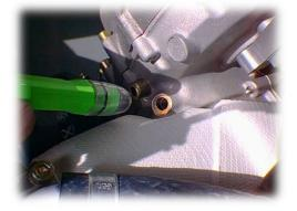
6. Remove the M8x20 socket head screw in the engine case right behind the gearbox. Use a flashlight in order to see where the V-grove for the locking pin bolt is. With the flywheel cover of, use a ratchet wrench with a 22mm socket and turn the crankshaft in the orientation of normal rotation until you see the V-grove in the crankshaft.
