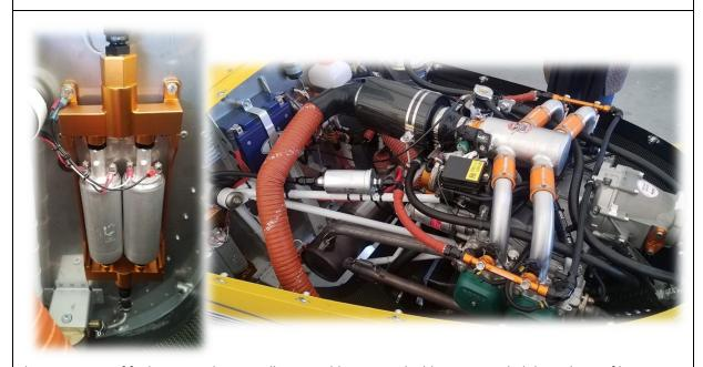
Showing wiring of fuel pump and EFI installation. Cold ram-air is highly remomended through a air filter.
