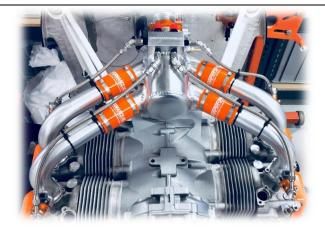
15. Alternative intake design when installed on engines with hydraulic propeller governor, DUC hydraulic actuator etc.
