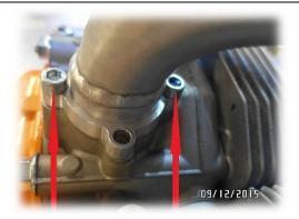
17. Install 2x M6 socket bolts in each of the four intake flanges. Tighten the bolts to **12NM**. Bolt lengths vary from intake to intake.
