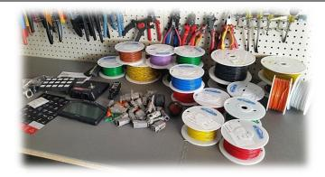
35. For the electrical wiring for the ECU chassis-lead, Pumps etc., ensure to use high quality TEFZEL milspec aviation grade tin plated copper wire. Do not use cheap automotive PVC cable. Remember, the wiring job is the most critical on the entire installation.
