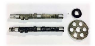
10. Both gears and the woodruff key, are now removed from the stock camshaft and is ready to be installed onto the performance camshaft.
