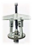
7. Pulling of the camshaft driver gear with the same 3-legged puller.
