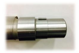
13. Gently tap the woodruff key into the new camshaft with a small hammer. Preferably, with a copper or brass hammer. Ensure it sits centered and with slightly nose down to make sure it enters the groove cut into the gear smoothly.
