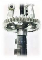
8. Ensure that the puller legs are all the way inwards to the camshaft.
