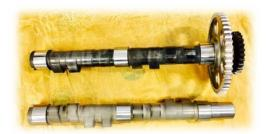
2. With the stock camshaft out of the crankcase, you see that the camshaft drive gear and the water pump gear must be pulled off, and installed onto the performance camshaft.
