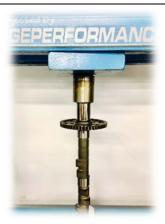
15. Use a suitable socket or make a sleeve on the lathe, and press the drive gear all the way down toward the mating flange on the camshaft using a hydraulic press. It may be good practice to slightly heat the gear with a propane torch and putting the camshaft into the freezer for 10-15 minutes. Ensure to slightly lubricate the gear and camshaft with engine oil before pressing the gear onto the camshaft.
