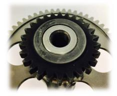
20. The gear face and the camshaft should be leveled.
