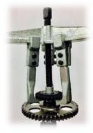
3. Securely fix the camshaft in a wise with soft aluminum or plastic jaws. Use a 3-legged puller to pull of the water pump gear. Using a M10 socket head screw with a solid steel washer comes handy when pulling of the gears. Slip the bolt in at the end as shown on the picture is section 5. Slowly pull of the gear. If you are unable to pull it off, apply some gentle heat by a heating gun or a propane torch.
