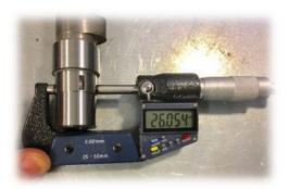
11. Always measure the camshafts 3 bearing areas and gear sections before installing the gears and the camshaft into the engine.
