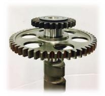
19. Water pump gear is now properly installed.
