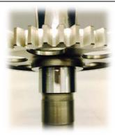
17. The gear shall slide all the way down to the mating surface on the camshaft.
