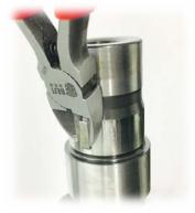
9. With the drive gear off, use a pair of cutting pliers etc., to gently remove the woodruff key.
