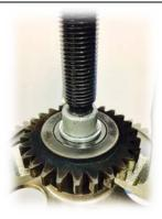
5. Here you can see the M10 socket screw and washer in place.
