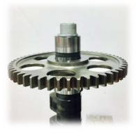
6. Now with the water pump gear pulled off, the camshaft drive gear is next.
