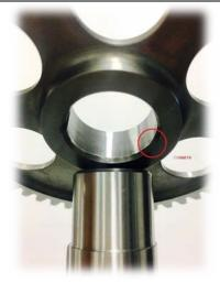
14. When installing the drive gear, ensure that the chamfered end of the gear faces down towards the camshaft.
