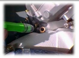
2. Remove the M8x20 socket head screw in the engine case right behind the gearbox. Use a flashlight to see where the V-grove for the locking pin bolt is. The groove will align with the hole when piston N° 1 is at TDC. With the flywheel cover off, use a ratchet wrench with a 22mm socket and turn the crankshaft in the orientation of normal rotation until you see the V-grove in the crankshaft.
