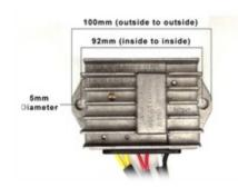
12. Install the regulator/rectifier on the firewall. The regulator must be installed in the engine compartment and cannot be installed inside the fuselage. If it for some reason must be installed inside the fuselage, and small 60x60mm or 80x80mm 12v fan must be used to prevent it from overheating and failing.
