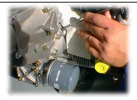
3. Install the locking pin bolt (Rotax part nr 240880) and tighten firmly.
