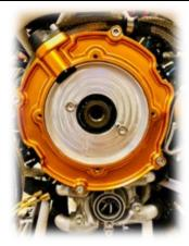
5. Now install the housing ring adapter with the 3x M6x25 bolts and the M6x60 bolt with the spacer at the lower left hole mating to the water pump housing. Insert the centering tool and orientate the notch so that it clears the crankshaft sensor. Apply Loctite 243 and torque all 4 bolts to 12Nm.
