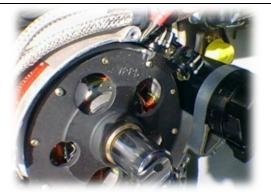
4. Undo the flywheel bolt. The bolt has normal right-hand threads. Normally a 50-60cm long socket wrench is required to loosen the bolt.
