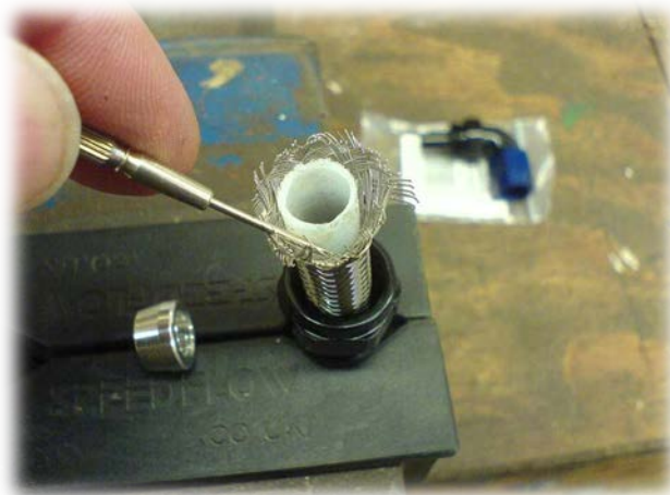
27. Spread the steel braiding to expose the PTFE tube.
