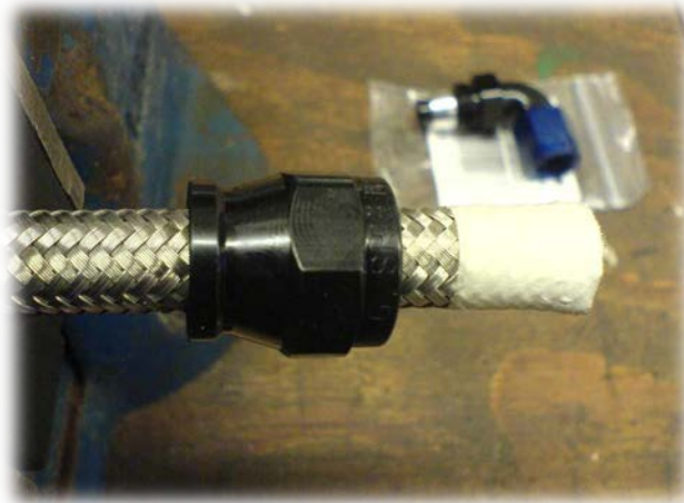
26. Sliding on the sleeve nut. Do this before you remove the tape.
