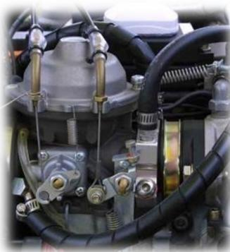
3. Now remove the LH/RH carburetors. Before you remove them, detach the air filters or airbox. Disconnect the choke and throttle cables. Disconnect the fuel hoses and hoses for coolant if you have carb heaters installed. Now loosen the Philips screw on the rubber socket flanges and firmly pull of the carburetors.
