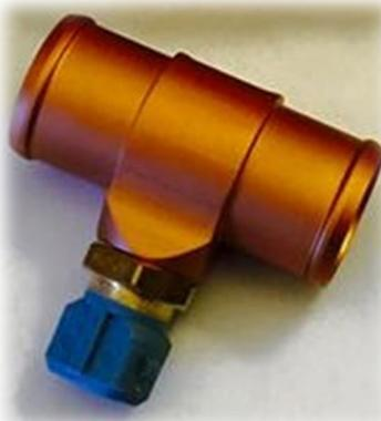
20. Cut the 25mm hose coming from the water collector tank, and install the coolant sensor adapter. It is usually convenient to use a 90° hose elbow. The “CLT” sensor is used for ECU engine temp feedback, mainly for cold or hot start, as well as enrichment when the engine runs hot.
