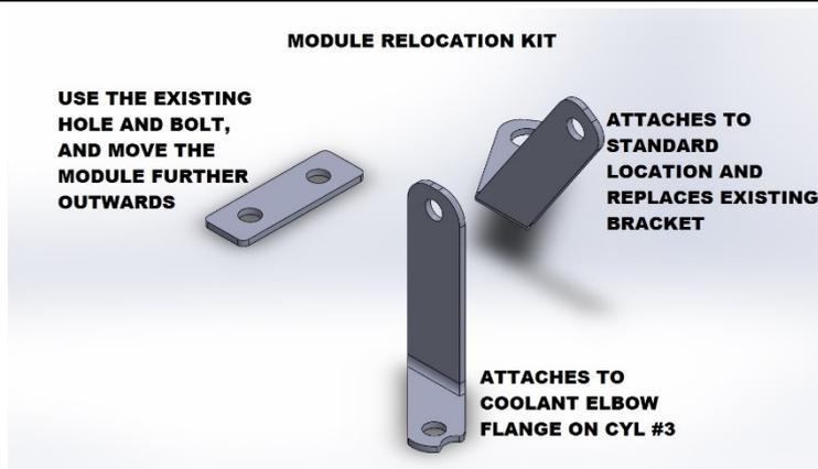
10. Install the provided relocation brackets for the ignition module. Various styles of brackets will come with the various intake designs or depending on is the ring mount is used (please specify when ordering). These may need to be modified or replaced in certain cases.
