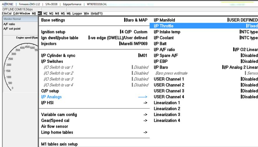
56. After starting the engine and setting the idle, go to M1, I/P Analogs and I/P Throttle. Now you can set the TPS idle and WOT limit. The TPS voltage is displayed in the picture as show in picture 54.
