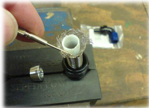
27. Spread the steel braiding to expose the PTFE tube. There are very practical hose spreading tools available from Summit-Racing, JEGS-Performance, eBay etc. #6 size.
