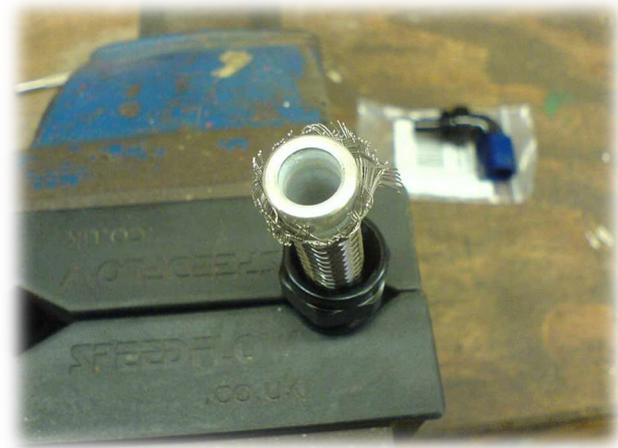
28. Install the olive insert ring onto the PTFE hose.
