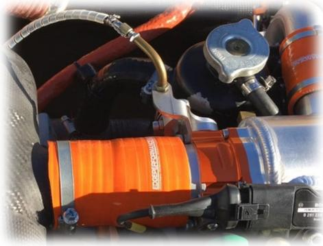
19. Use the 90° cable adjuster bend from the choke cable from you BING carburetors. Take the nut from the second bend so that you have two nuts and are able to clamp it onto the throttle bracket.
