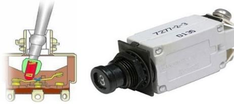
34. You will need 3x switches and 3x breakers in your panel. Skip the “optional” breakers. The breakers act as “short circuit protection” NOT as over current protection. That is why they are set so high. You don’t want the ECU to switch off in case an injector would fail and draw lots of amperage, or the fuel pump due to a clogged or frozen fuel filter.
