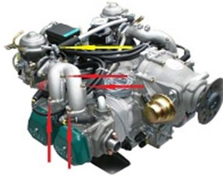
4. Loosen the hose clamp on each side that secures the balancing cross tube. Remove it from each intake manifold. Next, undo the 4x M6 socket head screws and remove the intake manifolds. Make sure to seal of the intake ports in the cylinder head with either a clean cloth, paper or a plastic plug as supplied with new engines in the exhaust ports. Replace the old intake O-rings (4pcs) with the new ones.
