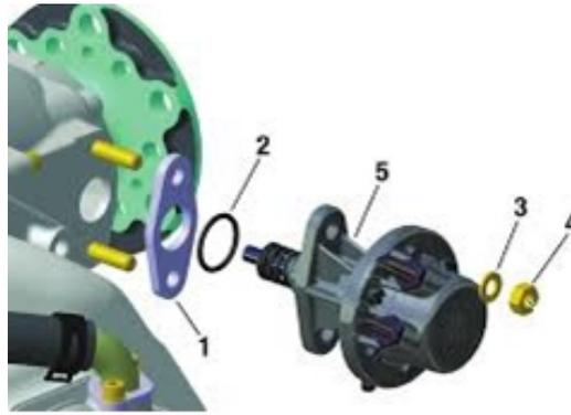
1. Remove the existing mechanical fuel pump. Start by removing the 6mm and 8mm fuel hoses. Remember to close the fuel valve before you start on this task. Next, remove the 2x M8 nuts and washers. Pull out the fuel pump and remove the isolator plate, gaskets and O-ring. Remove the M8 stud bolts by using a stud bolt extractor or simple by installing two nuts and unscrewing them.
