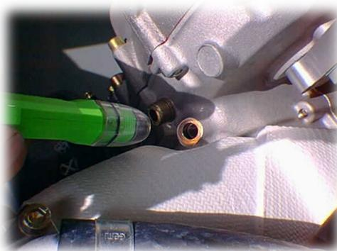
6. Remove the M8x20 socket head screw in the engine case right behind the gearbox. Use a flashlight in order to see where the V-groove for the locking pin bolt is. With the flywheel cover off, use a ratchet wrench with a 22mm socket and turn the crankshaft in the orientation of normal rotation until you see the V-groove in the crankshaft.
