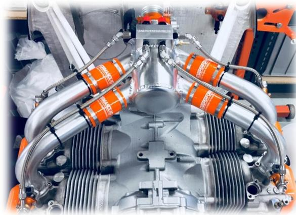
15. Alternative intake design when installed on engines with hydraulic propeller governor, DUC hydraulic actuator etc.
