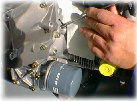
7. Install the locking pin bolt (**Rotax® part nr 240880**) and tighten firmly.
