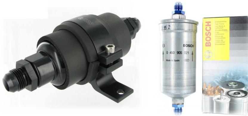
23. The post-fuel filter should be installed after the pumps. Note the arrow or in/out orientation indicating the direction of flow. Always try to install the filter in horizontal orientation. High flow, low restrictions or a gascolator is preferred prior to the pumps.
