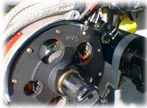
8. Now that the crankshaft is fixed, carefully apply some heat to the hex flywheel bolt with a heating gun or a propane torch. Perform extreme caution when using a heat source around flammable liquids. Take great precautions, and have a fire extinguisher nearby, just in case. Now apply a generous amount of force in order to undo the flywheel bolt. Normally a 50-60cm long wrench is required in order to loosen the bolt.
