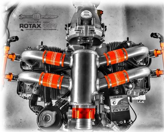
16. Install the 4-1 intake system on the engine. Ensure that the sealed off intake ports are free from any cloth, paper or plugs and insert new O-rings for the intake flanges. Orientate each intake flange with the mating flange on the cylinder heads.
