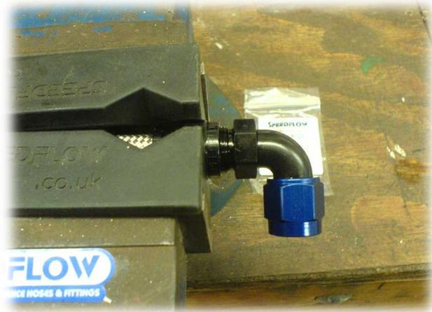
30. Clamp the assembly in the vise jaws and start to torque. Remember to lubricate the threads with some engine oil.
