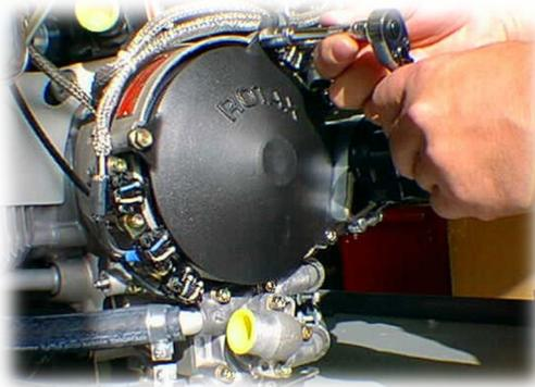
5. Remove the flywheel plastic cover by undoing the 3x 10mm M6 hex bolts.
