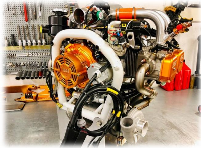
Secure the wiring harness from the back of the starter motor with a Adal clamp.
