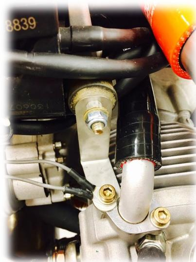
12. Terminate the two ignition grounding wires to the bracket bolt.
