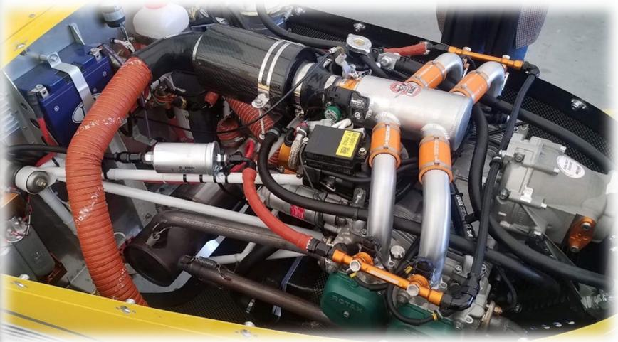
Showing wiring of fuel pump and EFI installation. Cold ram-air is highly recommended through a air filter.
