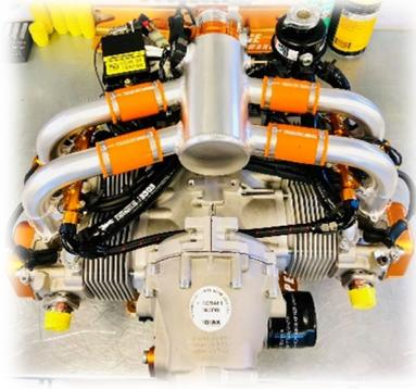
18. Cut the attached AN hose to length and make up the cross tube between the two fuel rails as shown on the picture above.
