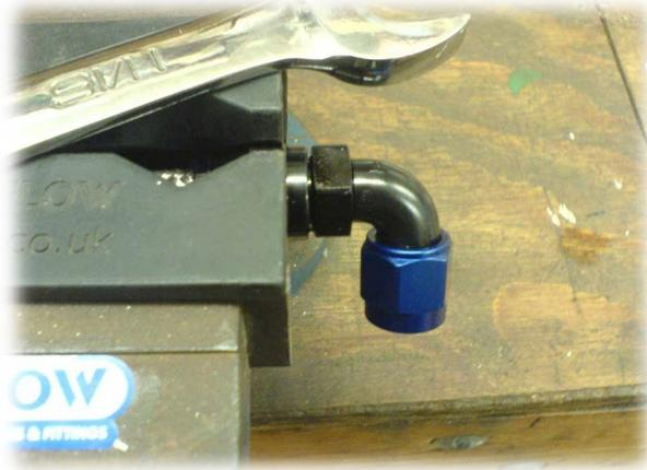
31. Keep torquing until the hose end and the sleeve almost mates.
