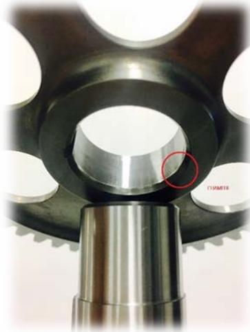
14. When installing the drive gear, ensure that the chamfered end of the gear faces down towards the camshaft.
