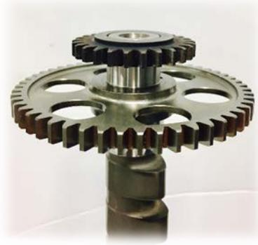
19. Water pump gear is now properly installed.
