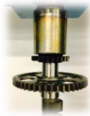
18. Next, install the water pump cam gear. Be sure that the gear enters straight. Slightly lube the cam and gear before pressing it onto the camshaft. Slight heat may be applied.
