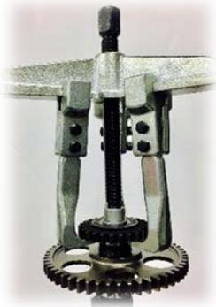
3. Securely fix the camshaft in a vise with soft aluminum or plastic jaws. Use a 3-legged puller to pull off the water pump gear. Using a M10 socket head screw with a solid steel washer comes handy when pulling off the gears. Slip the bolt in at the end as shown on the picture in section 5. Slowly pull off the gear. If you are unable to pull it off, apply some gentle heat by a heating gun or a propane torch.
