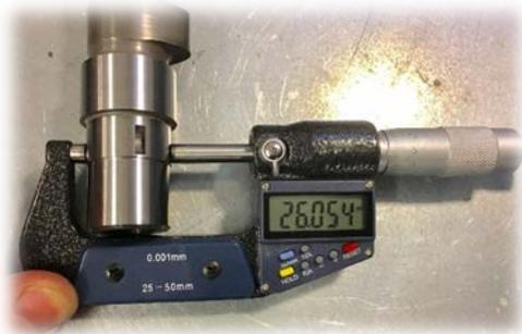
11. Always measure the camshafts 3 bearing areas and gear sections before installing the gears and the camshaft into the engine.
