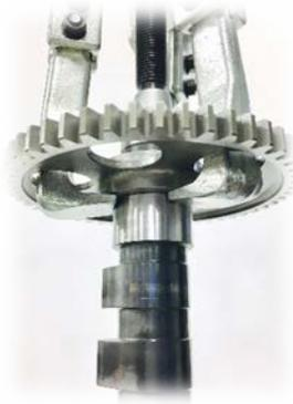
8. Ensure that the puller legs are all the way inwards to the camshaft.
