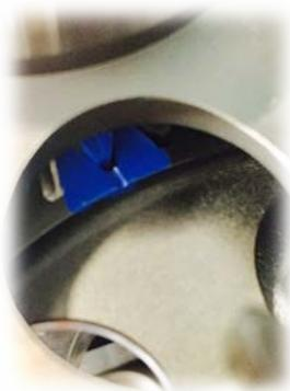
21. When installing the camshaft back into the case half 1/3, make sure to align the timing marks on the camshaft and crankshaft.
