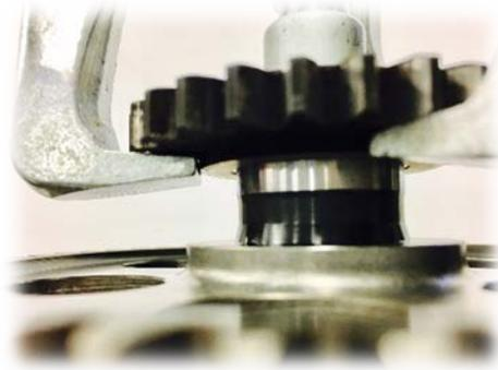
4. Make sure the puller “legs” are all the way in mating with the flange on the lower part of the gear.
