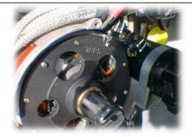
4. Undo the flywheel bolt. The bolt has normal right-hand threads. Normally a 50-60cm long wrench is required to loosen the bolt.
