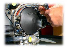
1. Start by removing the flywheel plastic cover by undoing the 3x 10mm M6 hex bolts.
