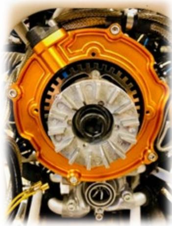
7. Install the trigger wheel and rotor assembly onto the M46x1 threaded section of the flywheel hub.
