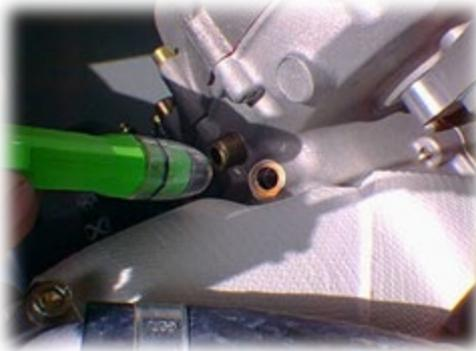
2. Remove the M8x20 socket head screw in the engine case right behind the gearbox. Use a flashlight to see where the V-groove for the locking pin bolt is. The groove will align with the hole when piston N° 1 is at TDC. With the flywheel cover off, use a ratchet wrench with a 22mm socket and turn the crankshaft in the orientation of normal rotation until you see the V-groove in the crankshaft.
