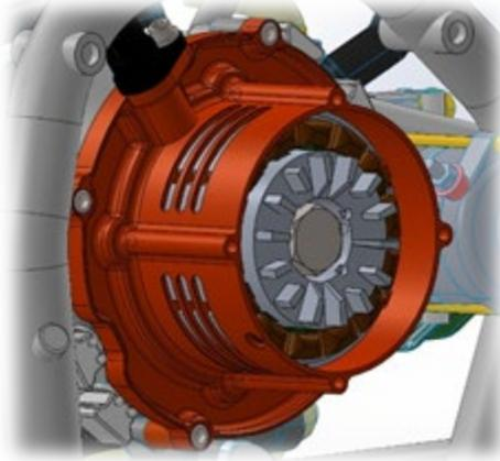
10. Next install the stator housing with the stator assembly seated all the way down to its seating flange internally. Ensure that the stator cables are exiting through the cable grommet hole.
