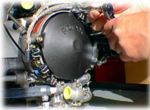
1. Start by removing the flywheel plastic cover by undoing the 3x 10mm M6 hex bolts.
