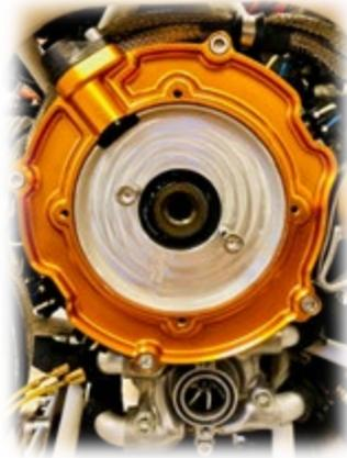
5. Now install the housing ring adapter with the 3x M6x25 bolts and the M6x60 bolt with the spacer at the lower left hole mating to the water pump housing. Insert the centering tool and orientate the notch so that it clears the crankshaft sensor. Apply Loctite 243 and torque all 4 bolts to 12Nm.
