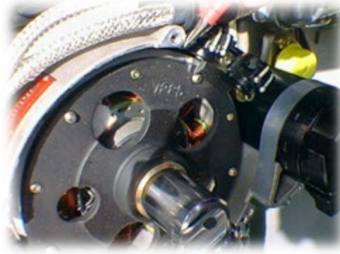
4. Undo the flywheel bolt. The bolt has normal right-hand threads. Normally a 50-60cm long socket wrench is required to loosen the bolt.
