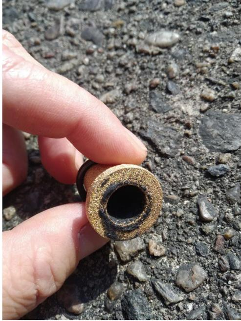
*Image 1. Clogged fuel filter resulting in very reduced fuel flow*
